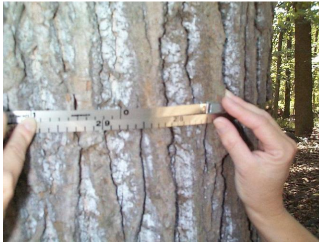
Measure to nearest tenth of an inch (29.2 inches in this example)
