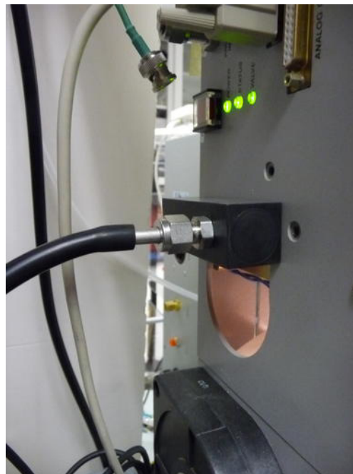
Figure 2. Closeup of modified nephelometer blower bypass block. Your nephelometer may have a blower installed in this location instead of a non-modified blower block. If so, remove the blower and detach the blower power cable. Insert the modified blower block in the place of the blower.
