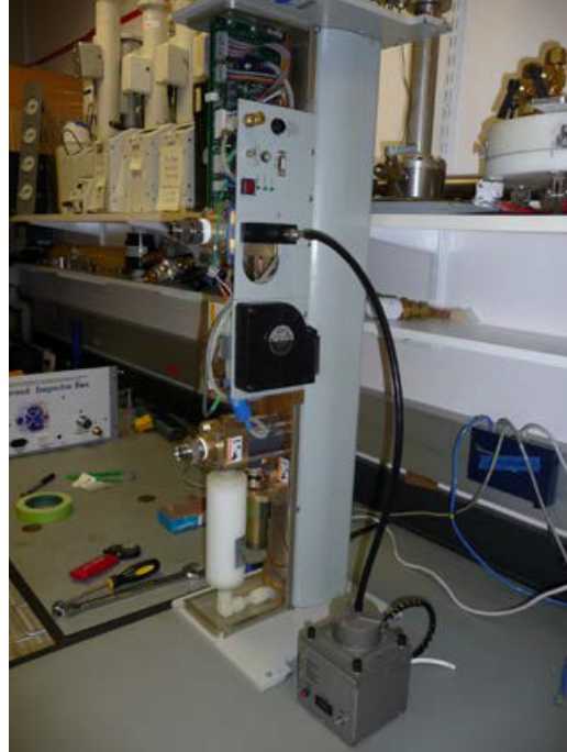
Figure 1. CLAP sampling from modified nephelometer blower bypass block. Blower block orientation is important – it should match the orientation in this picture – i.e., pick-off fitting should be closer to nephelometer sampling volume.
