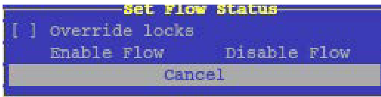
Figure 12. The "Set Flow Status" window is shown when the "Set flow override" option is selected. Selecting "Cancel" exits the menu with no effects. Selecting "Enable Flow" clears the user flow disable lock or all locks if the "Override locks" option is set. Selecting "Disable Flow" causes the CLAP to stop flow and sets the user lock. If "Override locks" is chosen, this sets a general lock.
