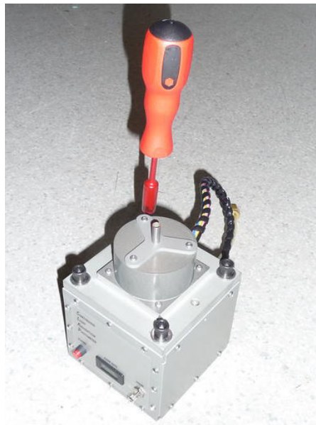
Figure 4. Top view of CLAP with top secured. To open CLAP for filter replacement, unscrew the four nuts on top using the torque driver.
