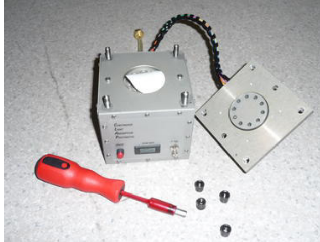
Figure 5. Top view of CLAP with top removed and clean filter inserted. Note the ten holes (eight sample + two reference) in the CLAP lid. The front panel contains a red pushbutton with internal indicator lamp, a display that shows the flow rate, and a manual needle valve that adjusts the flow rate.
