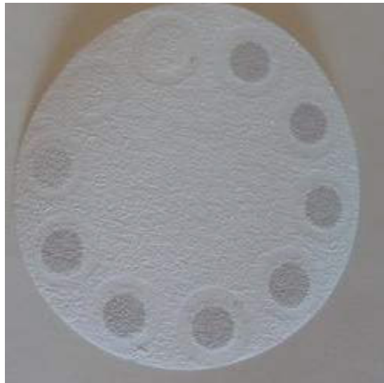
Figure 6. Photo of used CLAP filter. You can see the eight sample spots (1-8) and the two reference spots (R), which only measure filtered air. Reference spot R A is used for odd-numbered sample spots, and R B is used with even-numbered ones. On this filter, spots 1-7 were each sampled until the transmittance reached 0.7. The filter was removed from the CLAP when spot #8 had a transmittance of 0.84, which is why the #8 filter spot appears slightly lighter than spots #1-7.
