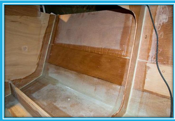
The picture here shows a plywood and fiberglass frame along the side and a plywood stringer along the bottom: strong, no beveling, no expensive wood, easy to build.
